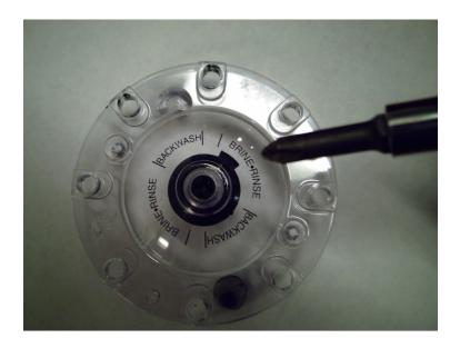
3. Insert the screwdriver into the recessed Phillips head in the center of the window. Be certain the cross pattern of the screw driver fully fills the head.
