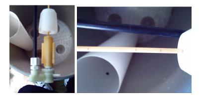
The float is adjustable by sliding along this rod. Careful examination will reveal faint reference lines along the rod. Note the location of your cup before cleaning it in case it is somehow moved in the process.
